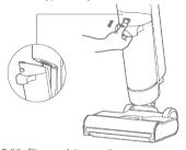
2. Pull the filter upwards to remove it.
